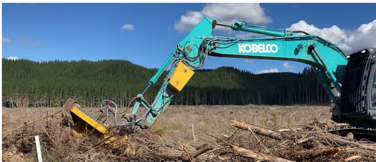
Figure 13. M-Planter machine operated by HA Fear Ltd. The machine head consists of a spot mounding implement and planting tube. The carousel holding the trees is visible on top of the planting head.
