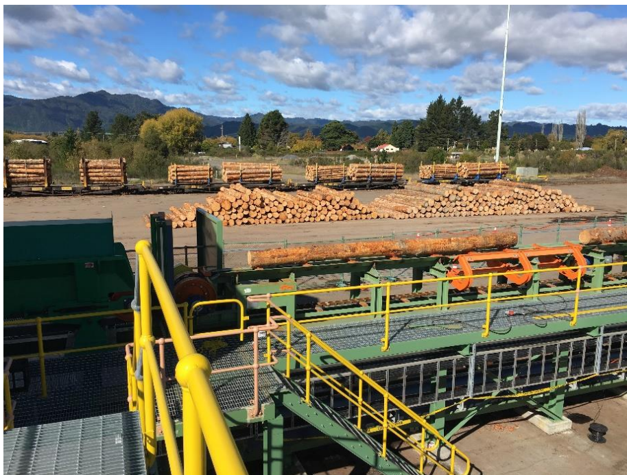
Figure 8. Logs exiting the de-barker at the MLY with rail wagons being loaded in the background.
