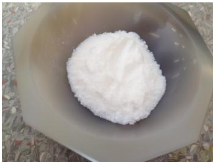
Fig. 8. Synthetic allophane made by Doreen Huang (PhD student) at Waikato University. Photo courtesy of Doreen Huang
