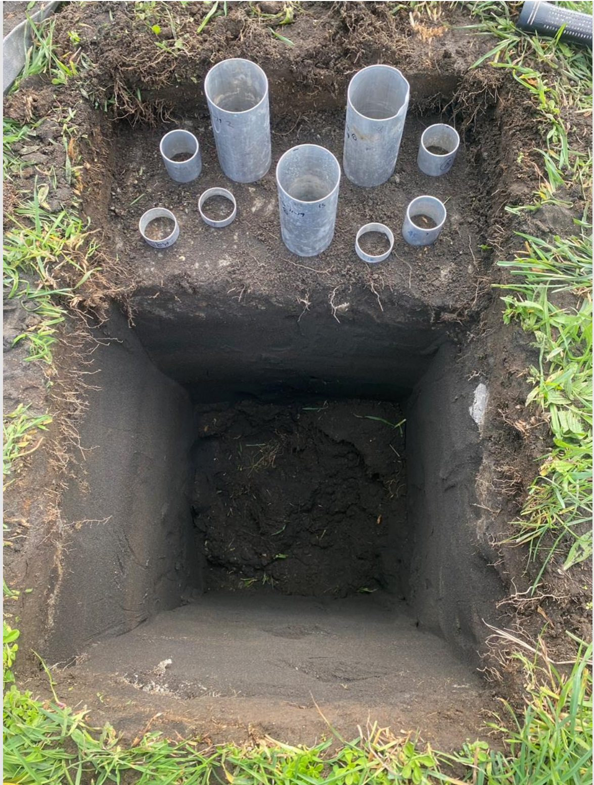
Figure 3. Layout of hydraulic conductivity, bulk density and retentivity cores taken from each horizon vertically down the soil profile.
