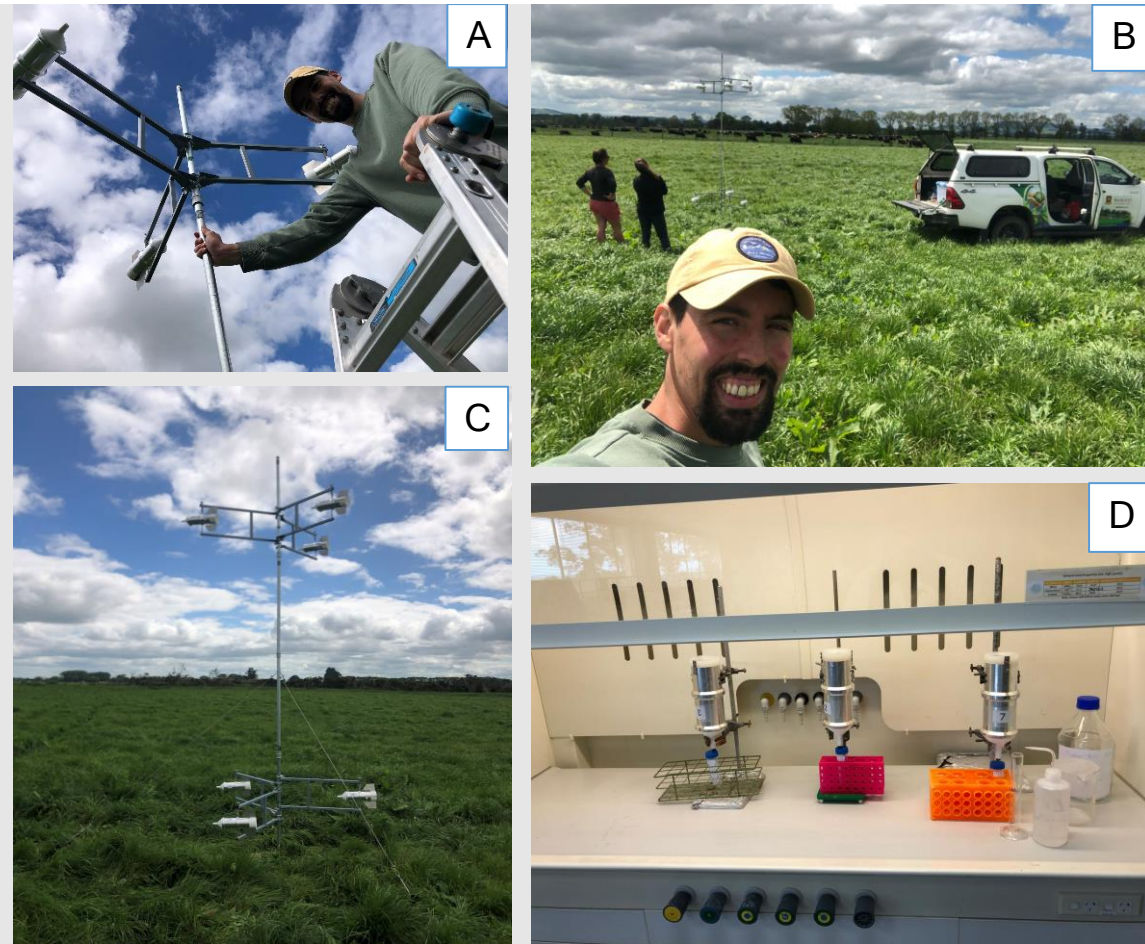
Figure 1 A. Franco, setting up the Leuning in triplicate at the top of one of the towers. B. Tower with Luening samplers at two heights near the milking cowshed. C. Tower with samplers at two heights in a paddock recently grazed by cows. D. Eluting samplers in the lab to measure ammonium.
