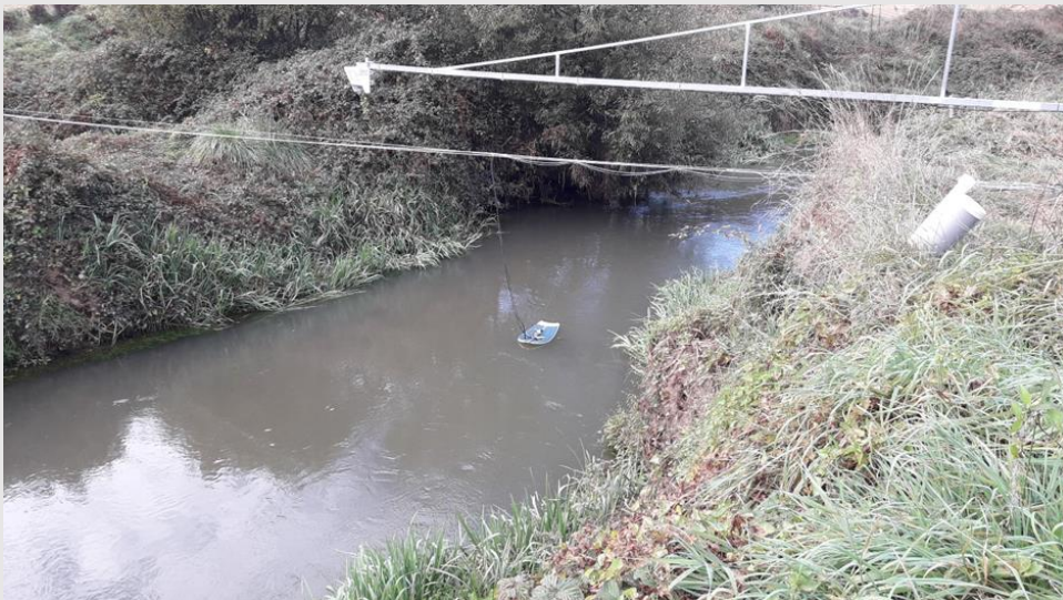
Figure 2: Waitapu stream measurement site, showing Geolux radar, new in-stream NICO location and previous NICO tube location, attached to the bank. April 2022.
