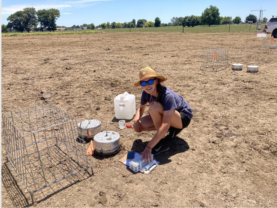
Figure 1: Summer research student Lee Boon taking gas samples from static chambers on a grazed area of the turnip paddock. The ungrazed turnips are in the distance.
