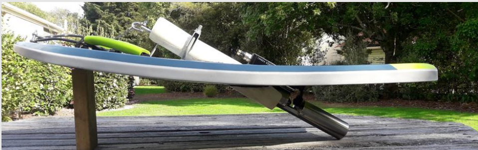
Figure 1: New boogie board deployment device with NICO nitrate sensor.
